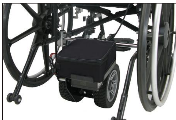
The Power Assist Battery Pack
